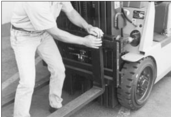
Figure 1: Removing the forks.
