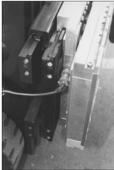
Figure 5: Assembling the load cell cable.
