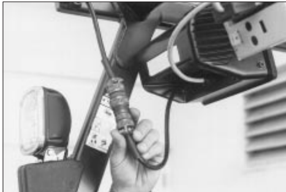
Figure 6c: Connecting the load cell cable.
