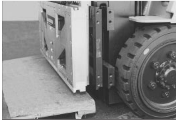
Figure 2: Loading the scale on the carriage.
