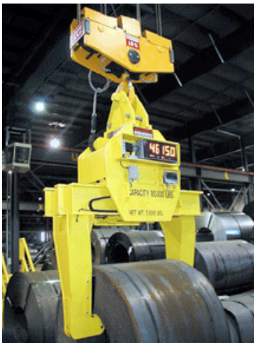
MSI CellScale technology used on this steel coil grab application.
